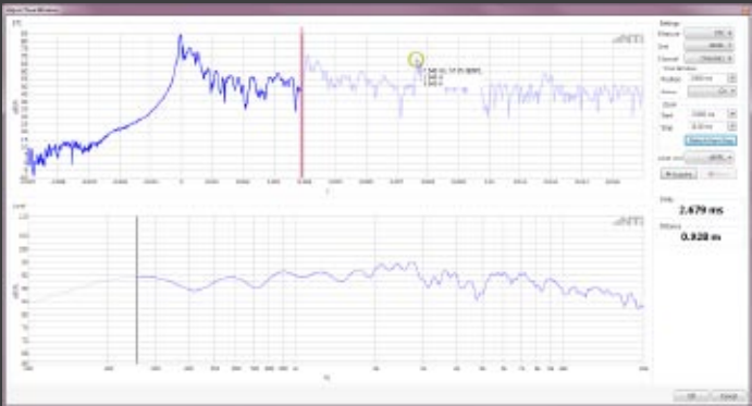
Time-gating for anechoic measurements
